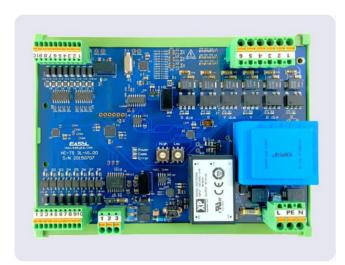
The interface for traffic lights LED HC-TS, developed and manufactured by *EASYsa*, is the ideal solution for a safe and remote control of traffic lights. The proper operation of the lights is guaranteed by the continuous current and voltage measurements and the feedback of the lights status to the control system
