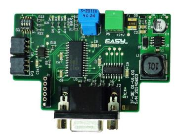
The PC interface for **IF-QE** incremental encoder developed and manufactured by **EASYsa**, is the ideal solution for the acquisition of incremental measuring positions.
